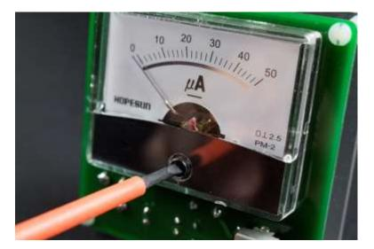
Do not force the screw to move, instead apply gentle pressure clockwise or counter clockwise to the screw while turning to adjust. It may take a few tries to hit '0'
