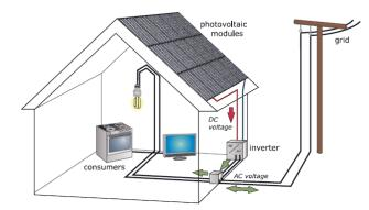
Figure 3. Principle of grid connected photovoltaic system.
