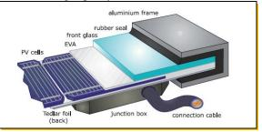
Figure 1. Structure of Photovoltaic Module [1]
