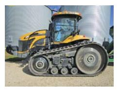
2012 Challenger MT765D: 8.4L, 6cyl diesel, 24" rubber tracks, (21) front weights, SISU Engine, 4 hyd., 2500+/- hrs., SN: AGCO765CDNCD1246.
