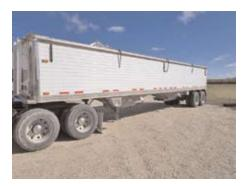
**2009 Timpte Super Hopper Trailer:** Ag hoppers, electric roll tarp, air ride, suspension dump, 11R-24.5 tires, outside aluminum/inside steel, LED lighting, SN: H4002 VIN: 9B118950, excellent condition.
