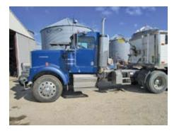
**2004 Kenworth:** W-900 B Model, C15 CAT, single turbo, Eaton 10sp. transmission, dual breathers, dual exhaust stack, headache rack, 411 rear end, 8 bag air ride, 11R-24.5 near new tires, 650,000 mi., SN: MBN23813
