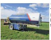
**1983 Progress Water** Tender: 3200 gallon, Power Pro pump, storage box, top or side fill, 22.5" tires.
