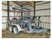
Travis Seed Cart: 4 box holder, easy load, 8 hp Honda engine, tandem axle, tool box, poly cup auger.
