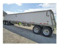
**2013 Timpte American AG Series Trailer:** 42 ft. air ride, aluminum inside/outside, suspension dump, LED lighting, 11R24.5 tires, SN H422, VIN: DB136940.
