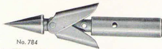
No. 784 DOUBLE BARBED HARPOON POINT Designed for attaching line at point. Lower point unscrews (as illustrated) for easy removal of fish, permitting arrow shaft to be backed out, instead of pulled through fish. Ferrule sized to slip over 5/16" shafts.
