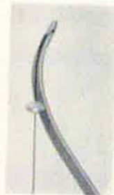
No. 672 TRUESPOT NOCKING POINTS Made of lightweight nylon tubes. Easy to attach to bow string . . . to reduce finger pinch and to provide a smooth, extremely accurate, hair trigger release. Enables a comfortable full three finger draw. Will not roll string, squash or deform on draw. Holds arrow in same position every shot. Can be removed from worn bow strings and used over and over.
