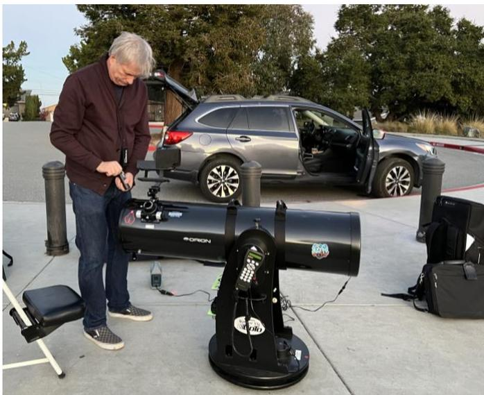
SMCAS Board Member Kevin Simpson sets up his Dobsonian 10-inch Orion GoTo. He usually sets it up with a Baader MaxBrite II binoviewer, with a pair of matching eyepieces. This allows people to use both eyes to view, which gives a slight 3D effect. The binoviewer has an attachment that boosts magnification of any pair of eyepieces by 1.7 times.
