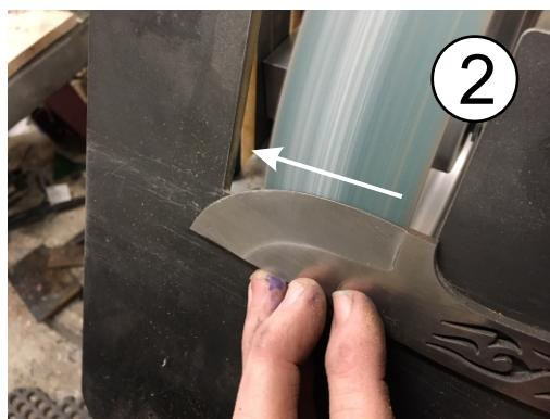
Maintain pressure to keep the blade flat while pulling it horizontally across the belt. As with flat bevels, it's very important to accurately grind evenly up to the scribed lines.
