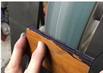
We recommend beveling a scrap piece of wood to confirm bevel width is set accurately.
