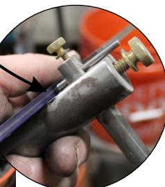
One trick of the trade when setting up the Tilt Table is to scribe a center line on a scrap of wood. Then test grind a bevel into the wood to see if the bevel is wide enough for the blade.
