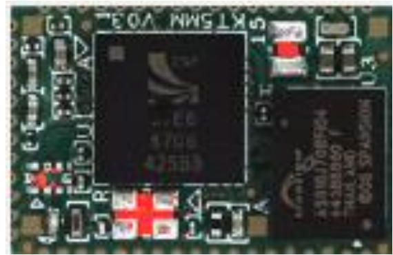
Figure 9: Missing SMT component detected in red color
