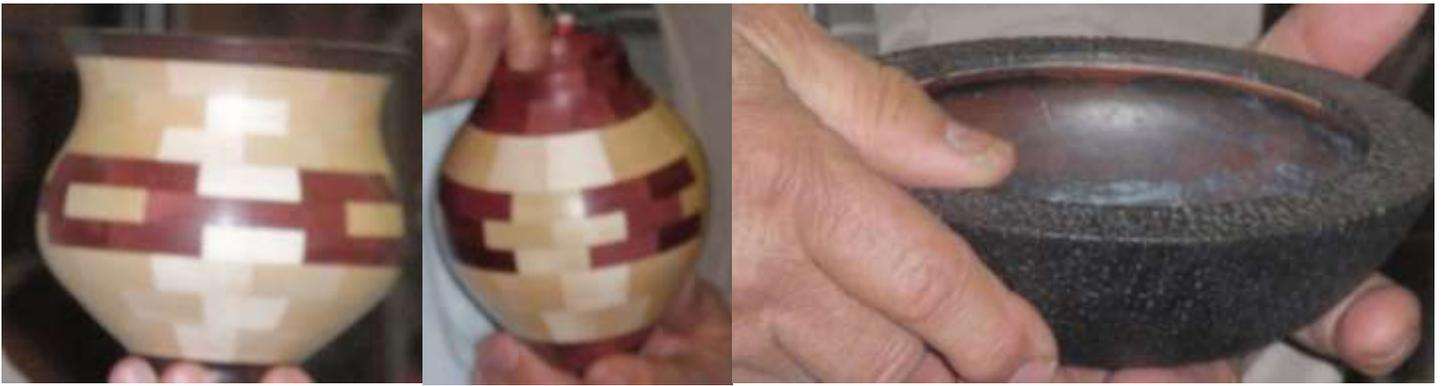
In the left photo, Pablo showed us a segmented bowl he cut, glued up and turned in which the rings were not centered properly. The next photo shows a variation in which the rings were aligned. He used Titebond in which the glue doesn't run for his glue up. He says it is "thick and quick".
