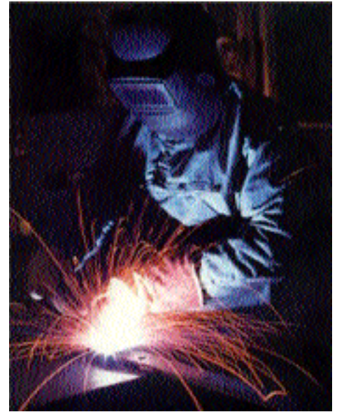
Welding in place: The very size and weight of large transit buses will not allow work piece turnovers, a constraint familiar to welders working on naval vessels or heavy construction vehicles. This fact mandates that a mechanic/technician be skilled in horizontal, vertical and even overhead welding when repairing or modifying the structure of a heavy vehicle.
