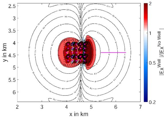
**Figure 2:** Relative change of the electric field in x-direction at 1300 m depth, caused by 25 boreholes with steel casings. The location of the boreholes is marked by purple asterisks and the purple line marks the position of the transmitter at surface. Colors show the ratio of the electric field with and without the steel casings. Black lines show absolute values of the electric field produced by the boreholes on a log-scale. Computations are for a frequency of 0.1 Hz.
