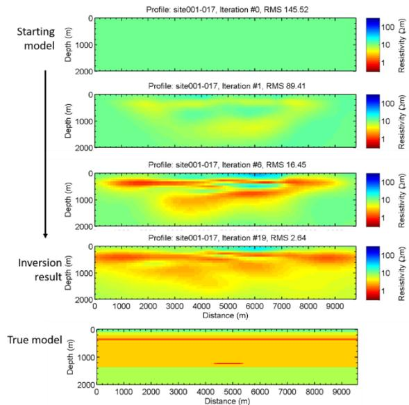
**Figure 3:** 3D CSEM inversion of synthetic data using field geometry for receivers and transmitters as shown in Fig. 1. From top to bottom: starting model, inversion results after 1, 6, and 19 iterations, true model.
