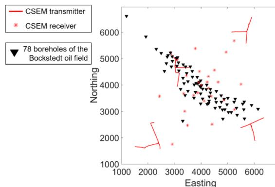
**Figure 1:** Survey layout for CSEM measurements in an oilfield in Northern Germany: red lines show positions of 4 three-phase current transmitters; red asterisks mark receiver positions; black triangles indicate locations of boreholes.
