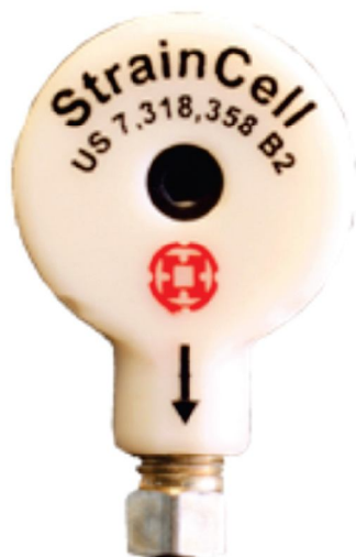
Figure 2. New-technology, bolt-on strain gauge
