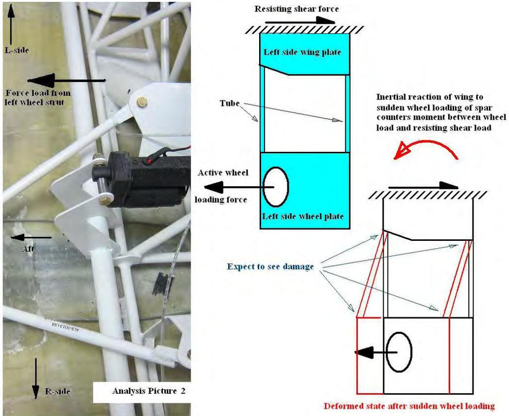
Figure 3: Analysis of Spar Box Structure, Picture 2
