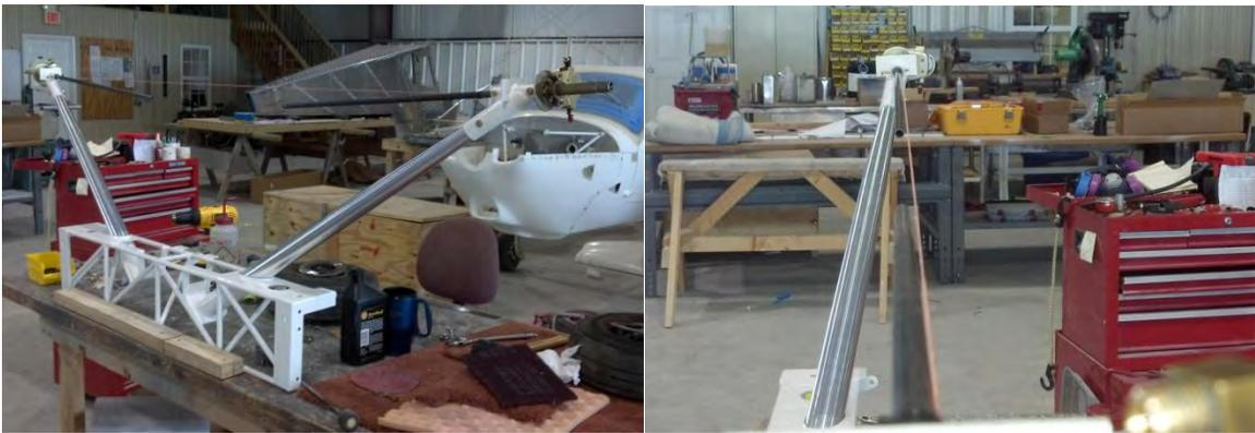
Figure 10: Setting the Toe (Factory pictures)
