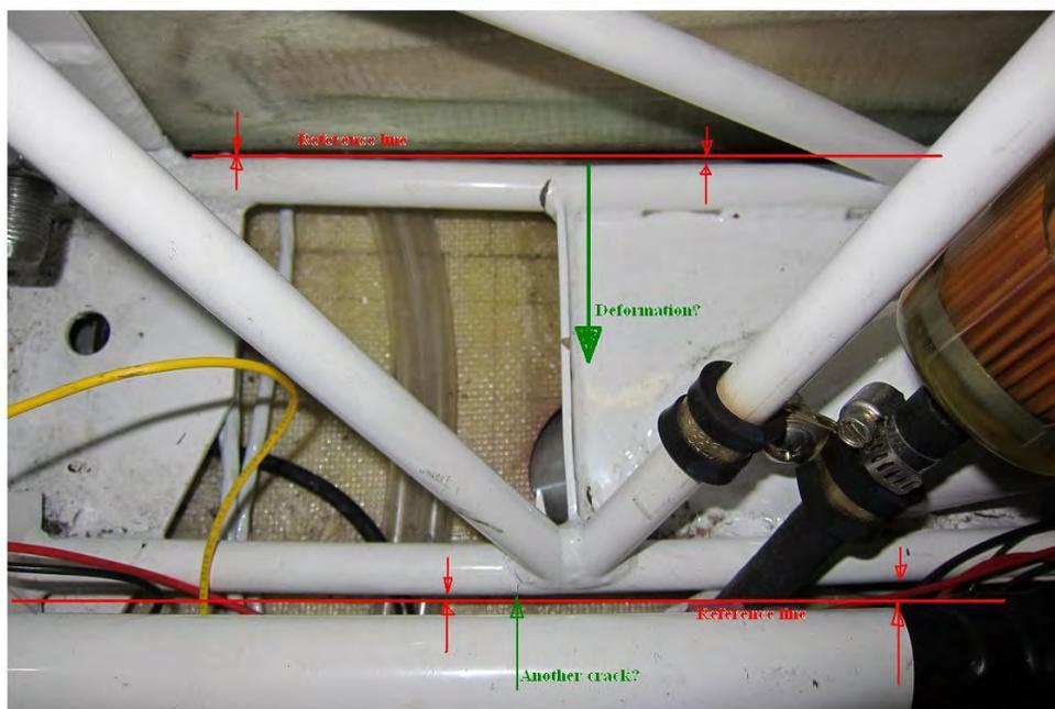
Figure 4: My Cracked Spar Box with Analysis
