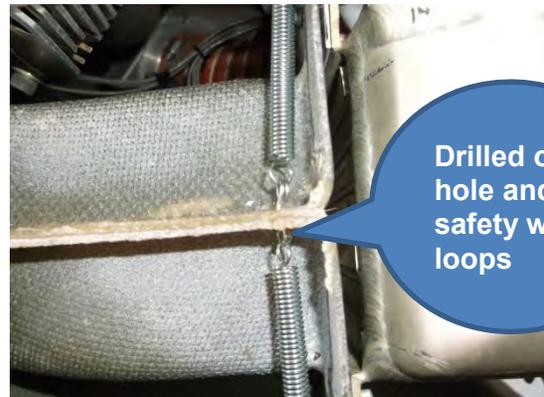
Drilled out hole and safety wire loops
