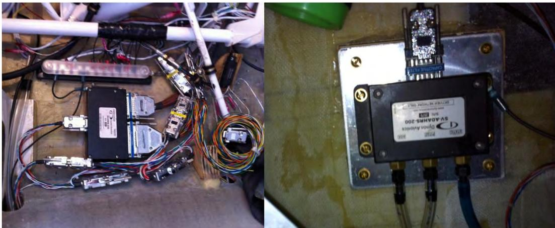
Figure 8: Engine Monitoring Computer (left) and ADAHRS (right).
