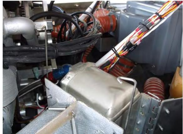
Next, I drilled a small hole in the top center seam of the fiberglass oil cooler inlet shroud and placed a piece of safety wire through the hole and terminated both ends of the safety wire in a double loop. I then took two small springs and hooked them onto the loops I just made. Finally, I bent each piano hinge pin back another 45 degrees (approximately) from the already bent 90 degree pin to be able to “catch” the other end of the spring.
