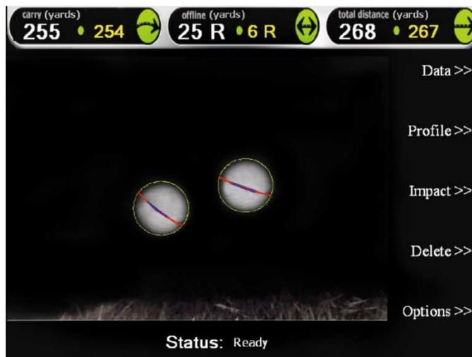
The '**Image**' view displays the image of the ball from the camera. The VectorX Launch Monitor uses a black line on the golf ball to measure the ball flight parameters; the line is indicated in red and blue by the software to validate how the shot was measured.
