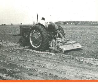
E-60 MODEL MIXING IN TREFLAN AND PREPARING A SEEDBED
