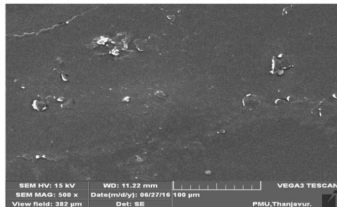
Figure 2: SEM image of copper adsorbed chitosan coated zerovalent iron Nano particle
