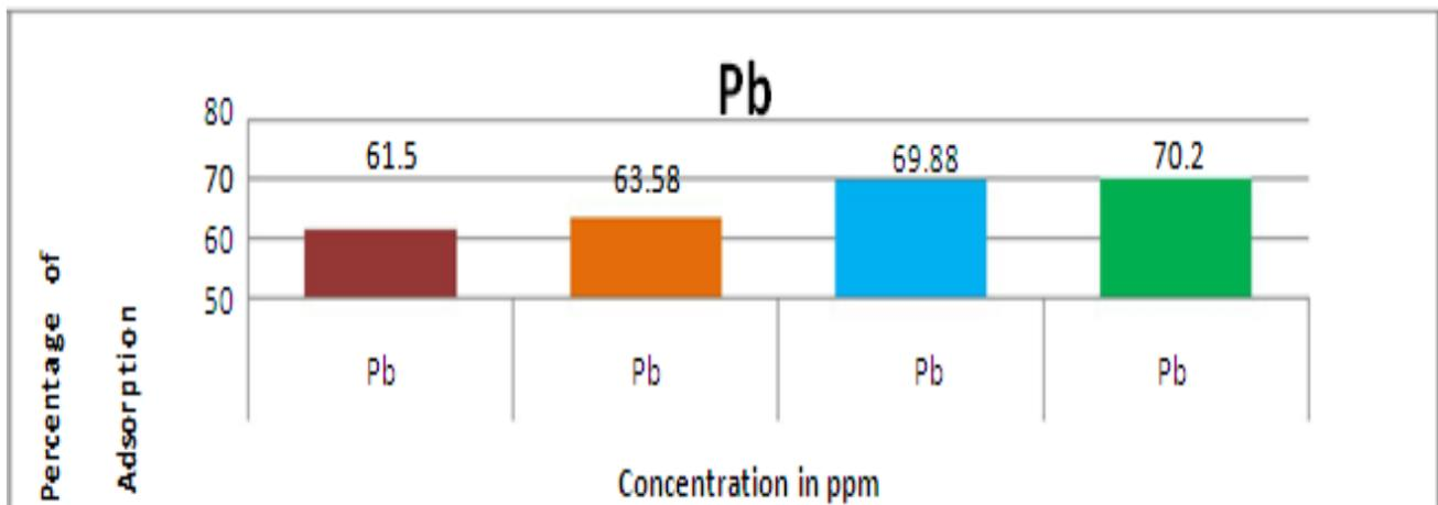
Figure 4 : Adsorption of Lead by Zerovalent iron -chitosan Nano particles at different concentration
