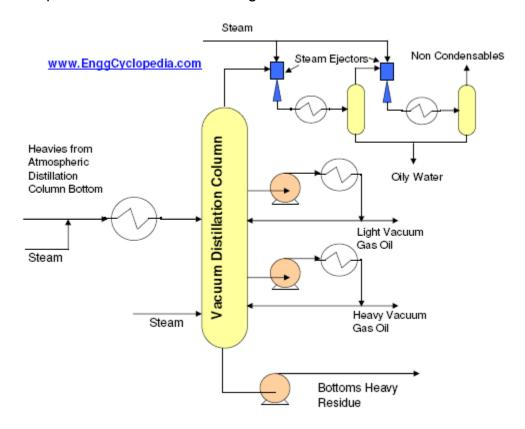
Dimensions for a distillation column vary considerably measuring from 3 to 48 feet in diameter. (O scale 1-12 inches) and 18 to 180 feet in height (O scale 4-40 inches). One rule of thumb is that the length to diameter < 30 so a 180 foot height necessitates a 6 foot diameter (O scale 40/1.5 inches).
