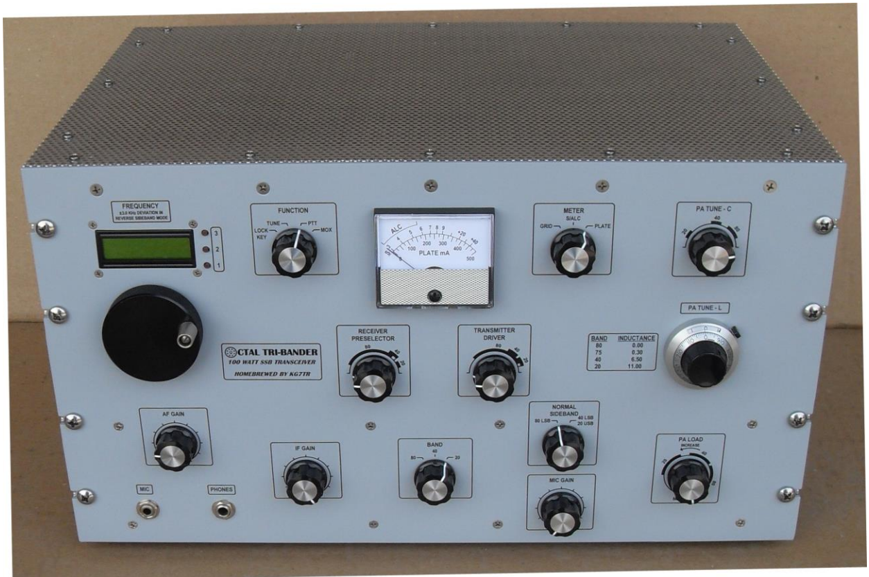
Figure 1: The Octal Tri-Bander Transceiver
