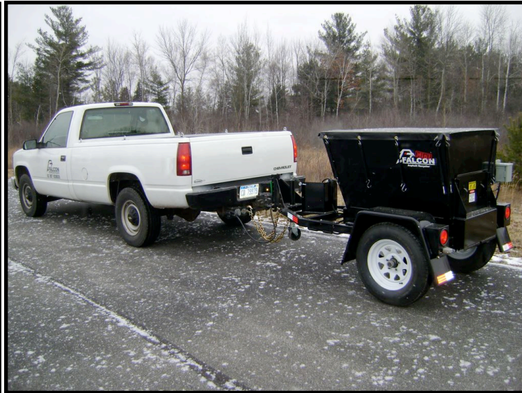
1 Ton MINI Trailer - Pickup Truck Length: 102" Width: 57" Height: 55"
