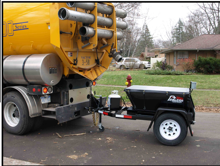
1/2 Ton MINI Trailer - Vacuum Excavation Truck Length: 102" Width: 57" Height: 50"
