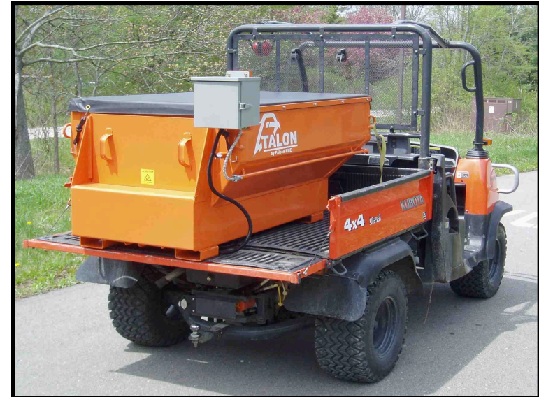
1/2 Ton MINI Slip-in - Utility Vehicle Length: 75" Width: 40" Height: 34"
