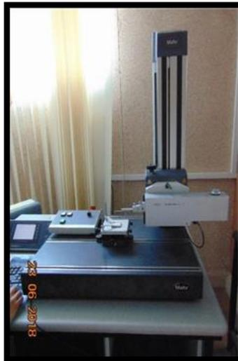
Figure (5) shows roughness-measuring device Mahr MFW-250
