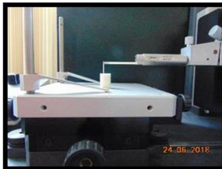
Figure (3) shows the sample during roughness measurement
