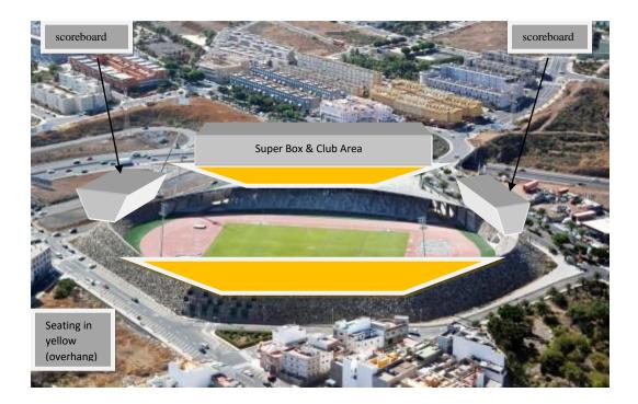
The above drawing illustrates the "buildup" model from a concrete base rather than the Old Pitt Stadium of "digging into the hill" concept. The issue is to lower the cost to build. **The New Pitt Stadium** may be able to provide covered seating as seen on the super box / club side of the field or open seating on the near side of this drawing (in yellow above).
