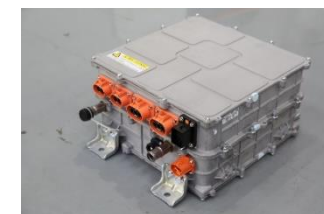
3-in-1 Controller Power Steering Brakes Low Voltage
