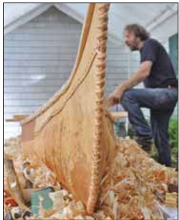
Canoe maker Steve Cayard checks the fit of a piece of hand-thinned wood destined for the bottom of the canoe. Below, the canoe has been created almost entirely with a small number of hand tools.
