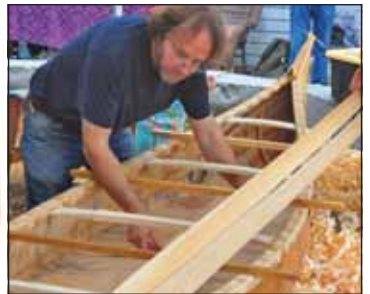
Canoe maker Steve Cayard checks the fit of a piece of hand-thinned wood destined for the bottom of the canoe. Below, the canoe has been created almost entirely with a small number of hand tools.
