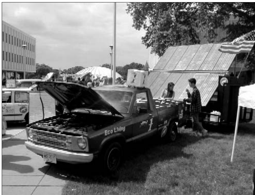
This Ford pickup, converted in 1981 by Jet industries, has a 30 Horsepower DC motor and GE SCR-1 controller.
