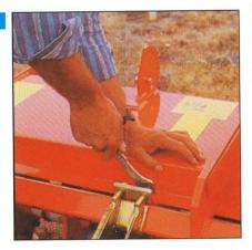
All models up to 1.80 m (70") may be operated centrally mounted or offset to the right hand side by simply repositioning the sliding clevis brackets. Offsetting enables the Rotavator to work close to the border line and even with the narrower models the right tractor wheel mark is taken out.
