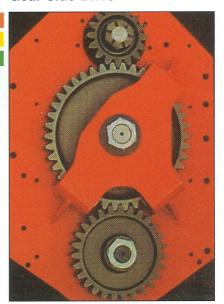
Gear side drives are for the more demanding cultivation applications, where higher horse power tractors are used. The gears, shafts and bearings are of heavy duty design as is the special "Y" idler gear support bracket which guarantees perfect alignment. The HR50 has two gear side drives and the rotor is driven from both ends: this provides long term reliability even when used in the most arduous of condition.
