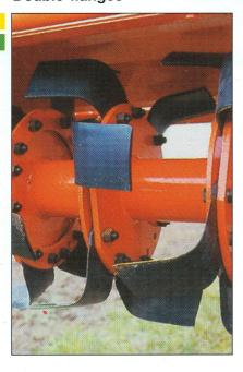
Standard equipment on the HR50 Rotavator and optional on the HR40. For heavy duty application the flanges create a clevis which double the shear capacity of the blade bolts and provides additional strength to the rotor flange.
