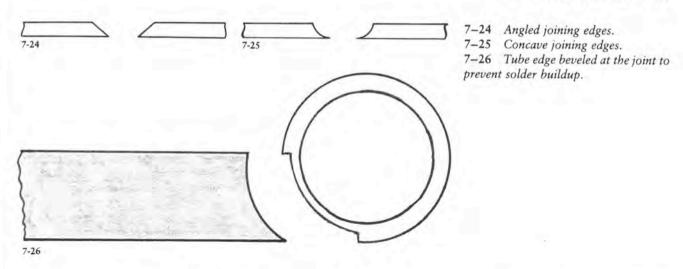
prevents a possible solder buildup along this area, which would make final fitting difficult.
