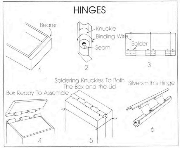
Fig. 153 Hinge Construction
