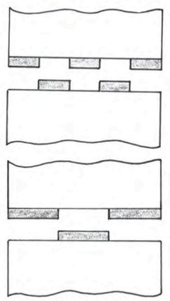
7-20 Sequence in which a three and five element hinge is soldered.
