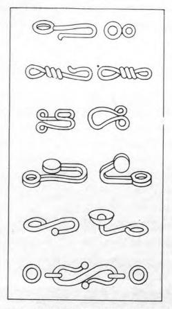
19-11 HAND-FABRICATED HOOKS MADE OF WIRE, USED FOR CLOSINGS.
