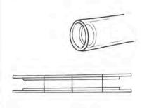
3. You will need several strips of flat springy metal. Watch mainsprings are best, but in a pinch, harddrawn brass, or nickel silver can be flattened out and used. Cut two or three pieces about an inch longer than the hinge. Slide these through and lock them with a pair of wedges, tapped into place.
