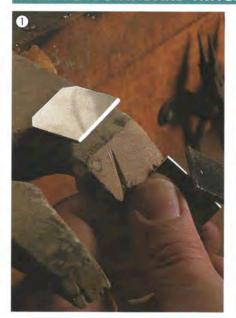
1 File the edges of the pieces at an angle; when laid together they should form a "V."
