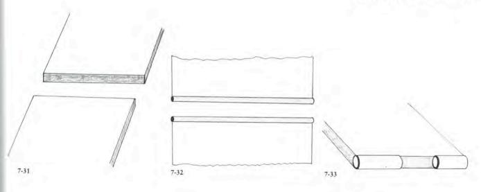
7-31 Joining edges prepared to accept tubes.
