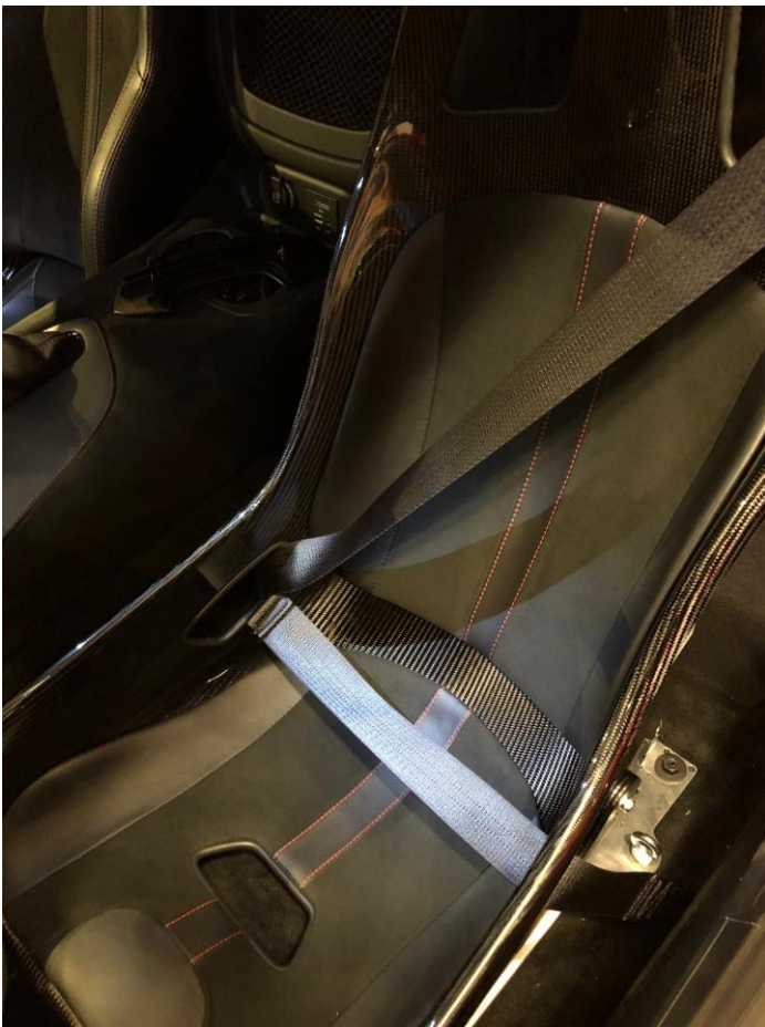
B7 Seat Installed with OEM Lap Belt Routed Through Seat
