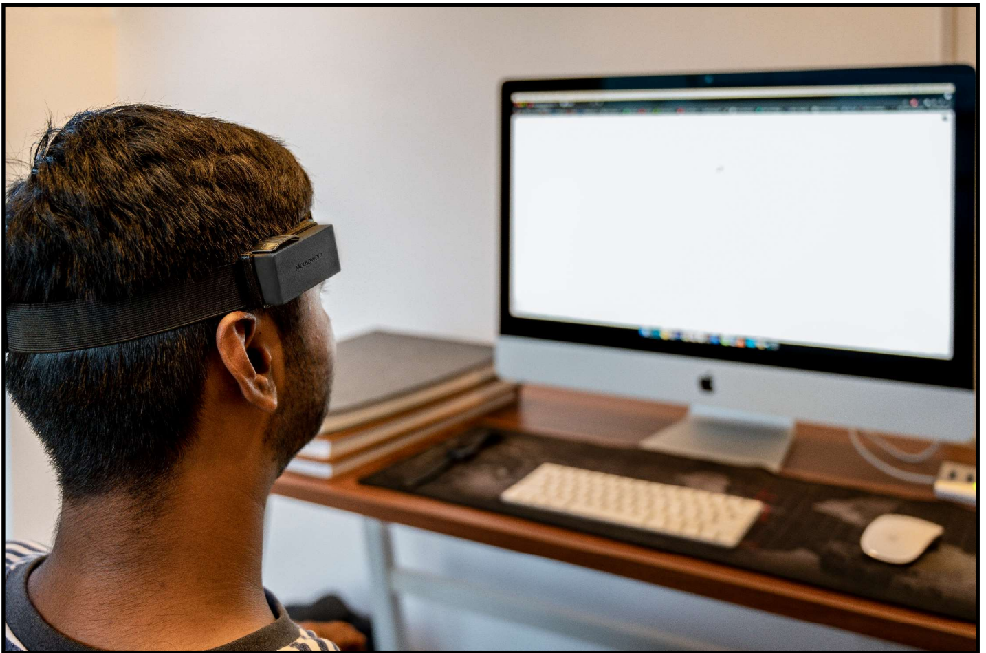
Picture description -A man wearing Mouseware above his ears on his head and accessing computer
