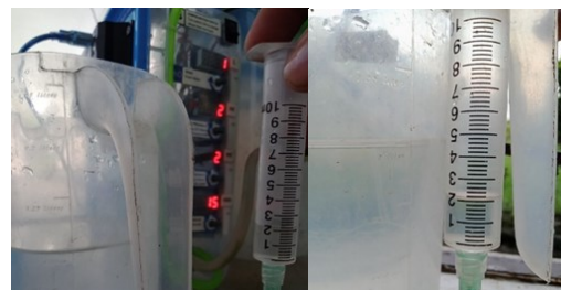
Figure 6. The Reliability test results of the device controller of Hydroponic Nutrient and Water Dispenser
