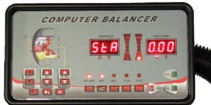
Quick & Easy Key Pad Data Entry for Static or Dynamic Precision Balancing
