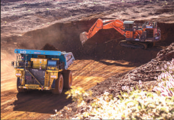
Rio Tinto was one of the first in the industry to adopt automation. Unlike its human counterparts, AHS trucks can run almost 24 hours a day, 365 days a year, only stopping for maintenance and refueling. By 2019, the company expects to have more than 140 AHS trucks in its fleet.
