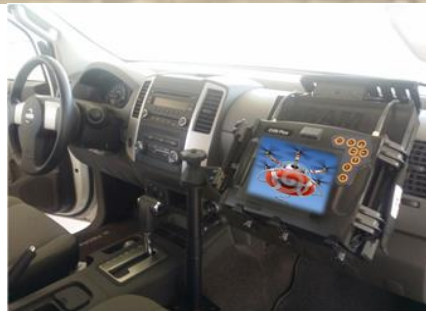
Portable Carry Viewer docked in Police vehicle for viewing video feed in real time
