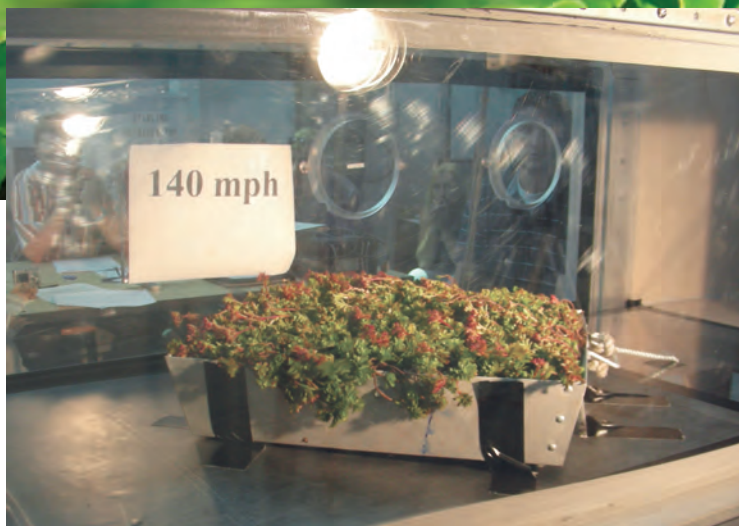
Test Specimen 1-3, a pre-vegetated module with 100 percent vegetative coverage, is positioned in the wind tunnel's test specimen bed.
