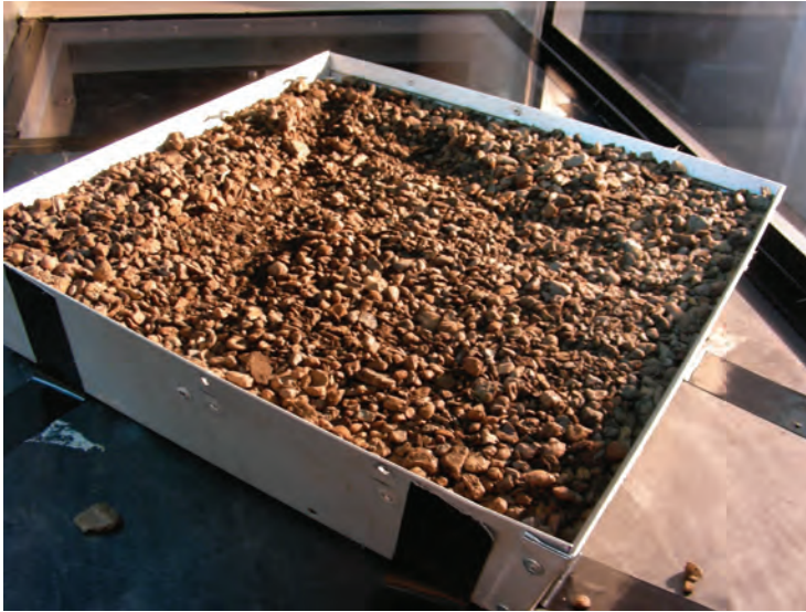
Test Specimen 1-5, which featured no vegetation and exposed growth media
