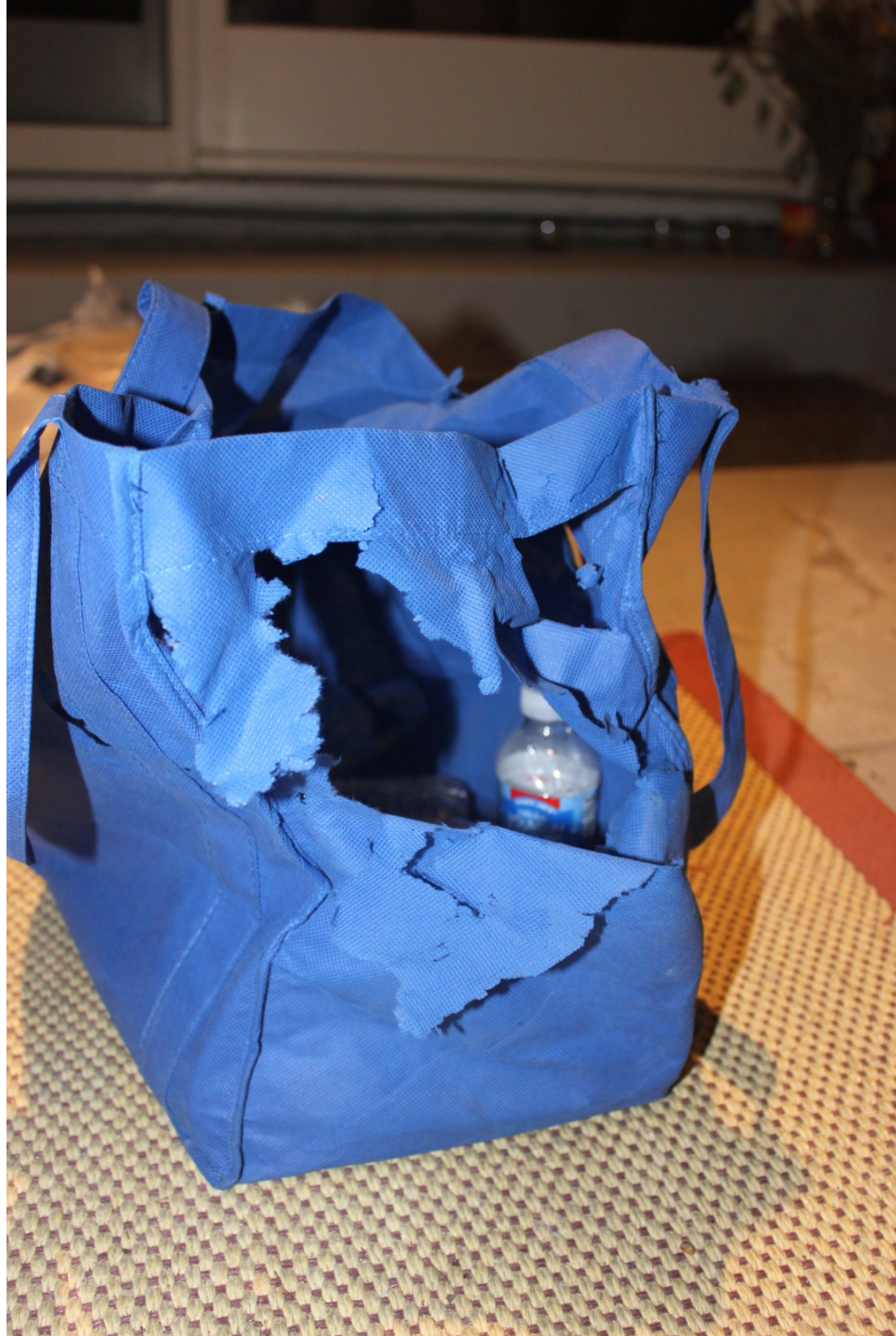
A polypropylene (PP) reusable bag after it has been washed in a washing machine. A PP reusable bag cannot be kept clean and reused more than a handful of times
