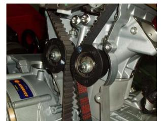
Install the belts, vertical cylinder first: bottom pulley first and work your way up.
