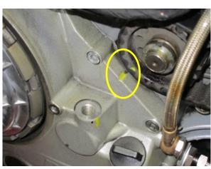
Align the marks on the intermediate shaft and the engine cover.
