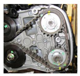
The yellow marks pictured on this horizontal cylinder are made on the pulleys where the valve cover gasket sets on the cylinder head. The three previous pictures show the pulley alignment at the "home" position. The markings will be necessary for reassembly when the belts have to be removed for replacement.
