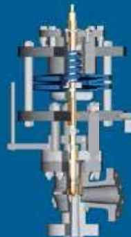
High-Pressure Steam Safety Valve in accordance with ASME I Si 9504-07
