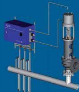
Controlled Safety Valve with PC 50
