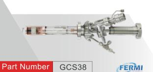
Atomic gas beams such as hydrogen atom beam are widely used for substrate treatment, this is usually done by introducing regulated gas flow through a heated metal capillary. The gas molecular would then dissociate at high temperature and inject into the vacuum.
