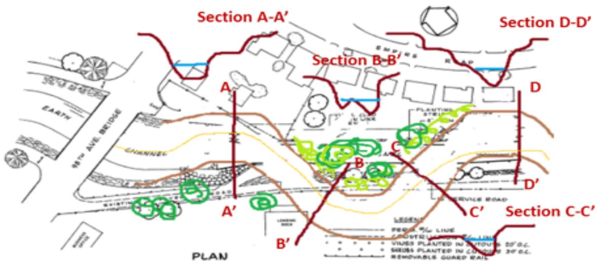
Figure 14. Altered design schematic with greater sinuosity and minimum channels
