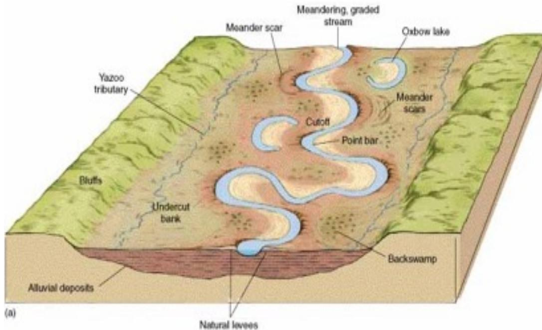
**Figure 8. Idealized Schematic of a Sinuous River and Floodplain**
