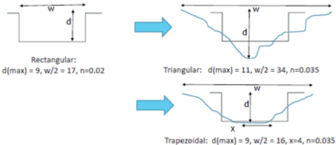
**Figure 15. Proposed Channel Modifications and Dimensions**
