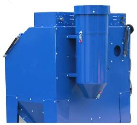
Then bolt on the dust collecting tank on the back of the cabinet. Connect the power cable from cabinet to the dust collecting tank.
