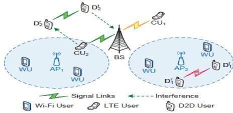
**Fig. 1 System model for LTE, D2D and Wi-Fi coexistence in both licensed and unlicensed spectra**
