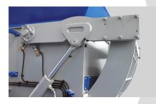
The G series shredders benefit from sturdy ram construction incorporating heavy duty guide bearings and universal couplings for reliable operation.
