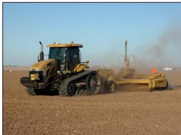
Figure 3.6c GPS-based Laser Leveling
