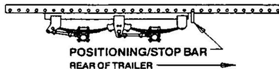
Sliders are equipped with a positioning/stop bar. Lock this bar in place immediately behind the slider whenever the trailer is in operation. (This does not apply to platform trailers when slider is in extreme rear-most position.)
