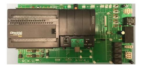
RCX is a drop-in control upgrade kit for Remstar vertical carousels. The system includes a PLC based machine interface board with pin-compatible connections to the existing control panel cables and components.
