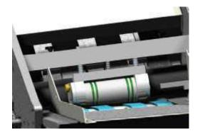
Indexing feed drum quickly rotates without the use of tools or technical adjustment
