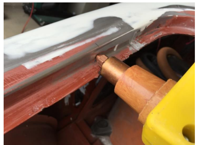
Closeup of Installed Trim Rivet
