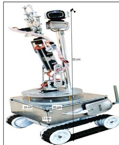
Fig. (9) Completed wireless mobile
