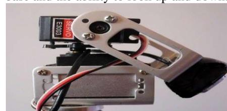
Fig. (4) Two standard servos mounted on top of each other for pan/tilt motion.
