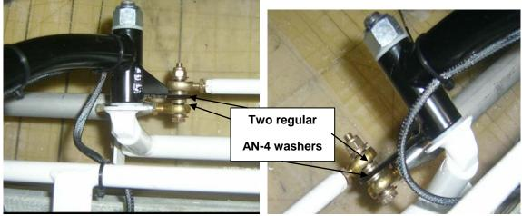
Note that there are two regular AN-4 washers on the inside of the rod end bearings next to the stick lower push pull tube attach point. Then on the outsides of the rod end bearings, there is one regular AN-4 washer and one large area washer.
