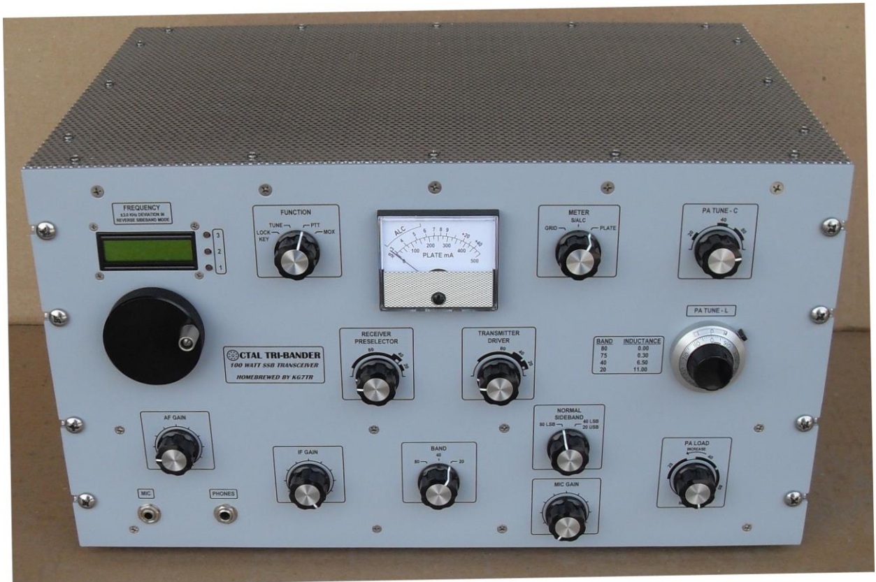
Figure 1: The Octal Tri-Bander Transceiver
